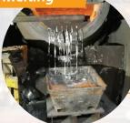
Prepared scrap is introduced into high efficiency furnaces that reach 1,400F.
